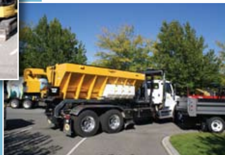
SANDER UNIT ON GRM 10.5 YARD SWAPLOADER ATTACHMENT
