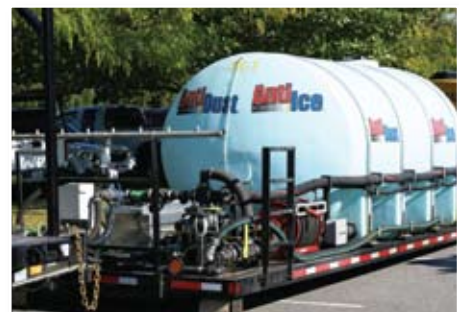
GRM SWAPLOADER ATTACHMENT WITH 3135 GALLON ANTIICE TANK ON 22' DECK
